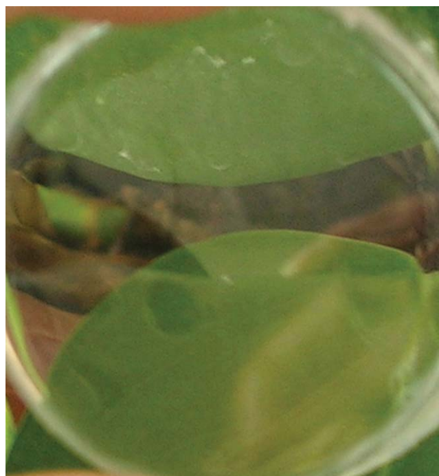
Figure 6 Photograph of the transparent film with 5 wt % ZnO (background: tree). [Color figure can be viewed in the online issue, which is available at www.interscience.wiley.com .]
